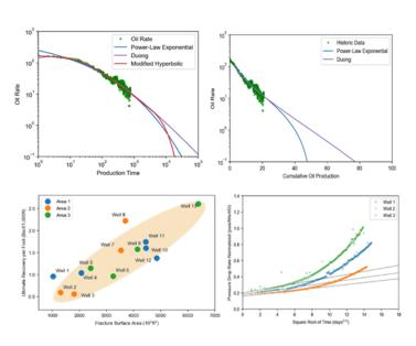
D&M applies a systematic methodology that combines diagnostic methods with analytical and numerical techniques to interpret and forecast well performance for unconventional reservoirs. This methodology assists with understanding what controls productivity, evaluating completion and stimulation effectiveness, and providing recommendations regarding well length, well spacing, hydraulic fracture spacing, etc.
